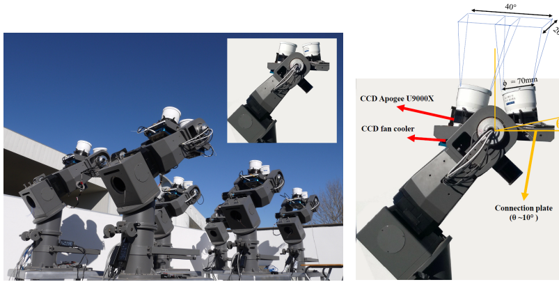
Fig. 1: ( left ) The mini-GWAC telescope farm, located at the Xinglong Observatory, includes 6 mounts and 12 Canon 85/f1.2 cameras. ( right ) Each mount is equipped with 2 cameras with a field of view (FoV) of 20^\circ \times 40^\circ for a total FoV for the whole system of about 5000 sq.deg (about 1/4 of the Northern sky). The image cadence is 15 seconds.
