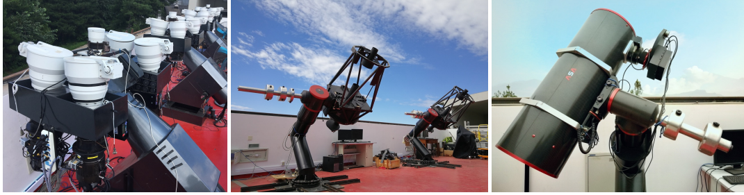
Fig. 9: (Left) The GWAC observation system in its test bench at the Xinglong observatory. For O3, it will be composed of 4 mounts. The total FoV of such configuration is about 2000 sq.deg. The imaging time resolution is 15 sec for single frames. (Center) Two GWAC-F60 telescopes (60cm) are used to quickly confirm GWAC optical transients and perform deeper follow-up observations if needed. (Right) A 30 cm telescope (GWAC-F30) will be also used during the O3 campaign (FoV = 1.8^\circ \times 1.8^\circ ).
